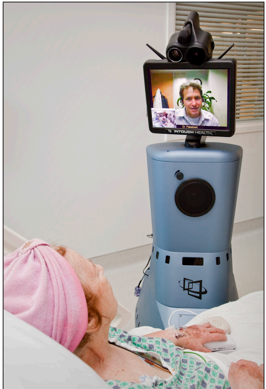
Dr. Palestrant, visits a Neuro ICU patient using the RP-7 robot, which can be driven right up to the bedside.
